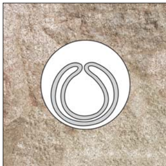
Original cross section shape of The GONLEX friction bolt when inserted into the drill hole.
